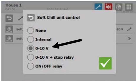
Select **0-10 V** so that the chill unit can be connected and controlled by an external DOL 31 fan speed controller.
